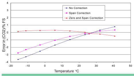
Temperature compensation corrects for temperature error in the detector.
