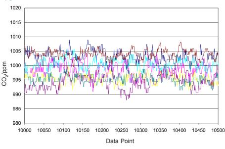
Excellent stability and resolution at 1000ppm CO<sub>2</sub> for the IRC-A1 is achieved by better design, not by using more expensive components.
