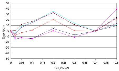
Custom linearisation is not necessary with the IRC-A1. Using universal linearisation constants, repeatability between cells is very good, allowing easy implementation.
