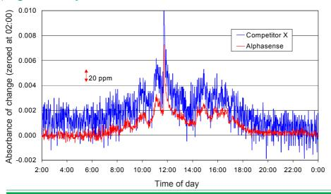
Comparison of resolution of IRC-A1 (red) and competitor's 20mm diameter NDIR cell (blue).
